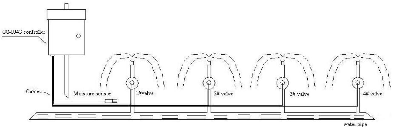
The next diagram shows the “Timer Control” mode. The moisture sensor would be used as a rain sensor; it cannot be installed near an irrigated area, must out and can be moistened by rain.
