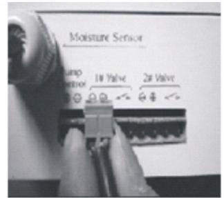
Then plug the terminal back in the controller where it came from. Make sure latching/DC valve connects to terminals with +/- sign, AC valves with AC power connect to switch terminal with no +/- sign. No errors tolerated.
