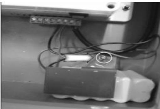
Disconnect the battery; remove the battery bracket, if necessary.
