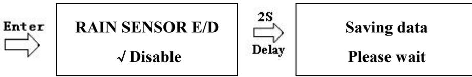
When the system is run under “Timer Control” mode with rain sensor enabled, the controller will check the rain sensor before opening the valve. The valve will only be opened when the current moisture level is lower than the set rain control sensitivity.
