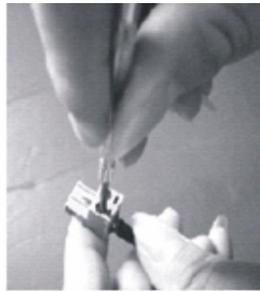
Reference +/- sign on the terminal, red wire to +, black wire to -, connect the valve to the terminal. (If no +/- sign, then either way is OK.)
