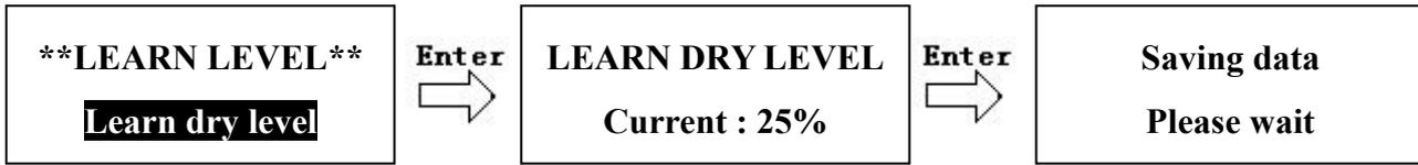
Current moisture will be shown, this is the present value collected by the moisture sensor, push “Enter”, this new moisture level is learned as the new set dry control level, replacing the old one, and returns to the previous menu. Pushing “Exit” will not save the new data, and returns to the previous menu.
