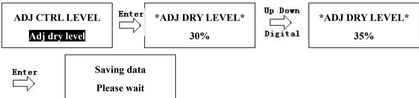
The display will show current setup value, the cursor will flash at the value position. User can enter the number, or push up/down key to adjust until reaching the desired %, then push “Enter” to save new value, and return to previous menu, or push “Exit” to exit without saving.
