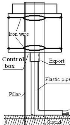
Or bound to a post. Using soft tube to protect sensor and valve cables
