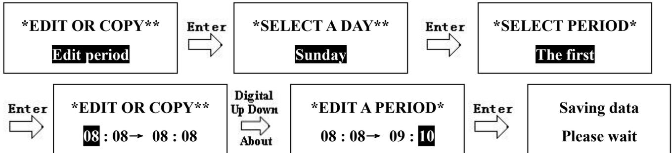
Lock out period has a beginning and ending time selection, during the lock out period, there is no irrigation except manual irrigation. The lock out period only functions under moisture control mode, not for timer.
