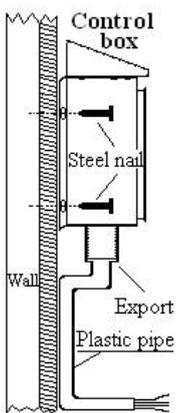
Install the box on a wall by using nails or bolts. Orient the solar panel towards Sun. Using soft tube to protect sensor and valve cables
