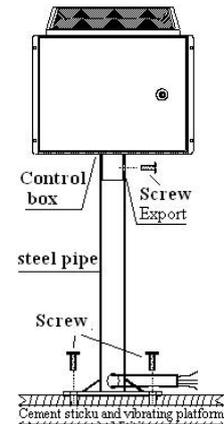
Or make a stand alone steel tube frame to support the controller box, and protect the sensor and valve cables.
