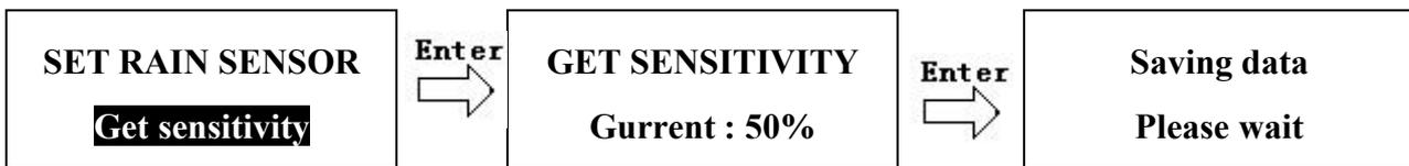
Learn rain sensor sensitivity means the controller learns/remembers one moisture percent level as standard to judge if there was rain. In “Timer Control” mode, the moisture sensor is used as a rain sensor. If the current moisture level is lower (drier) than the setup moisture level, then there was no rain, otherwise there was rain, and the controller will not open the valve.
