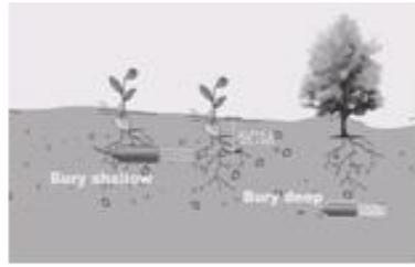
Find a representative location to dig a hole, then bury the sensor horizontally to the ground at some depth according to plants. Then pat the soil tight to make sure the soil fills the sensor probe
