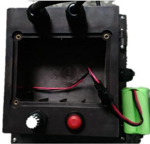
**Third Step:** Put the battery into battery box, cover back the battery cover and fix it use screws, as following picture.
