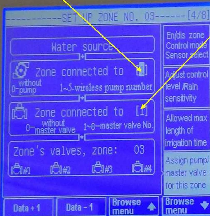
**1. Push function key browse into “Assign pump/master valve for this zone”**
